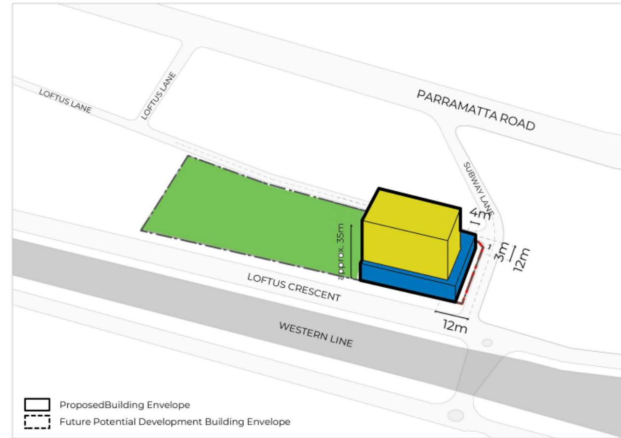
2. MASSING OF PROPOSED 11 STOREY TOWERS IN ACCORDANCE WITH BUILDING HEIGHT RECOMMENDED BY PARRAMATTA ROAD URBAN TRANSFORMATION STRATEGY REPORT.
