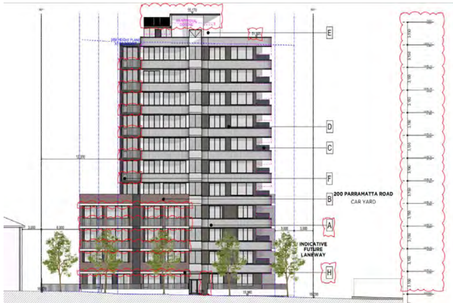
Figure 4: Proposed Bridge Road elevation plan showing increase in building height to 39.17m
