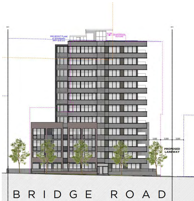
Figure 5: Approved DA2016/170/2 Bridge Road elevation plan showing maximum building height of 37.9m
