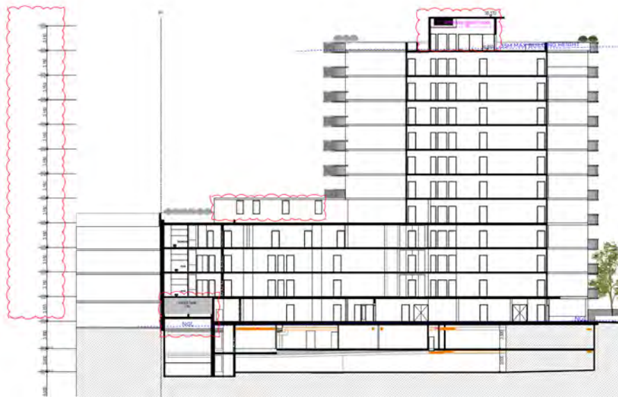
Figure 2: Proposed section plan showing 3.15m floor to floor height to accommodate NCC requirements for services and habitable 2.7m floor to ceiling heights.
