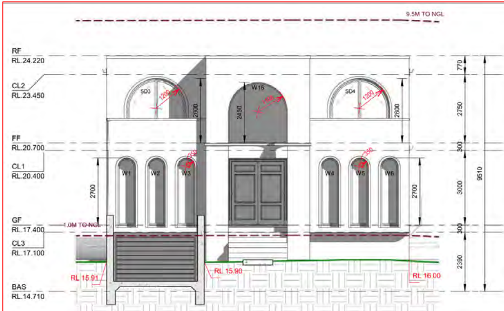
Figure 9: Refused Northwest (Front) Elevation
