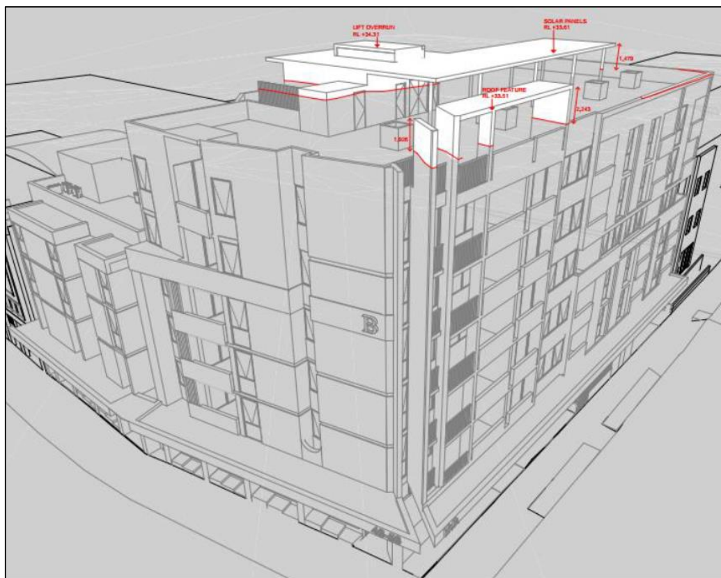
Figure 22: Diagram illustrating the aspects of the building that exceed the 22m building height development standard. Source: Fuse Architects
