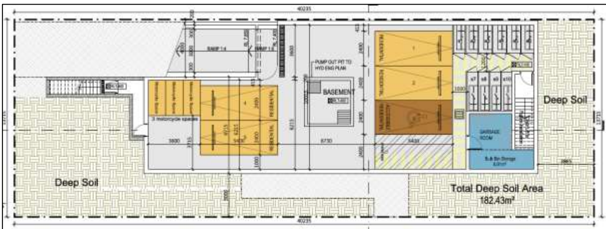
Figure 5: Approved basement floor plan
