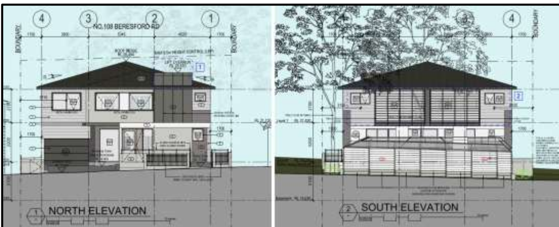
Figure 7: Proposed north and south elevations – note proposed lift overrun
