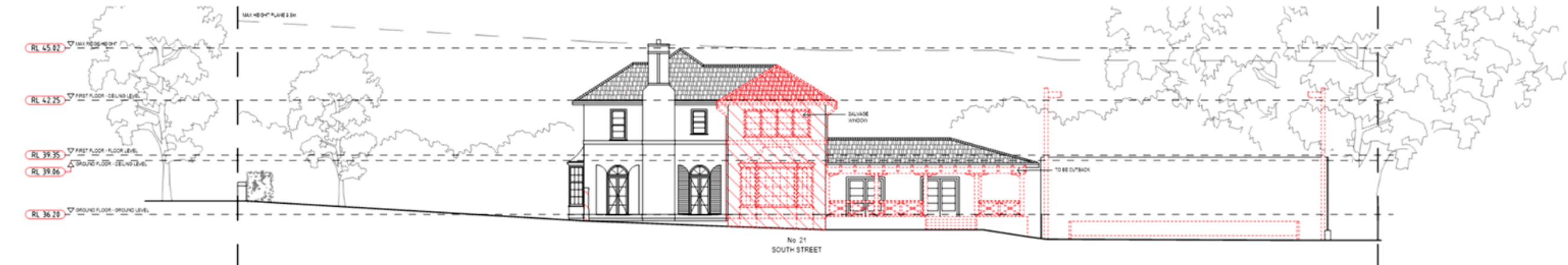
03 NORTH ELEVATION EXISTING + DEMOLITION - 1:200
