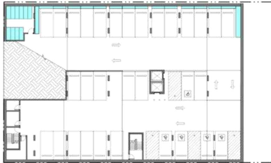
1 STORAGE PLAN - BASEMENT LEVEL 3 1: 200 @ A1
