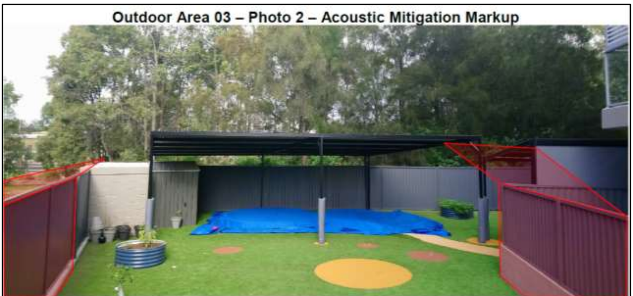
Figure 9: Proposed acoustic barriers and roof structure as recommended in the revised acoustic report facing east.
