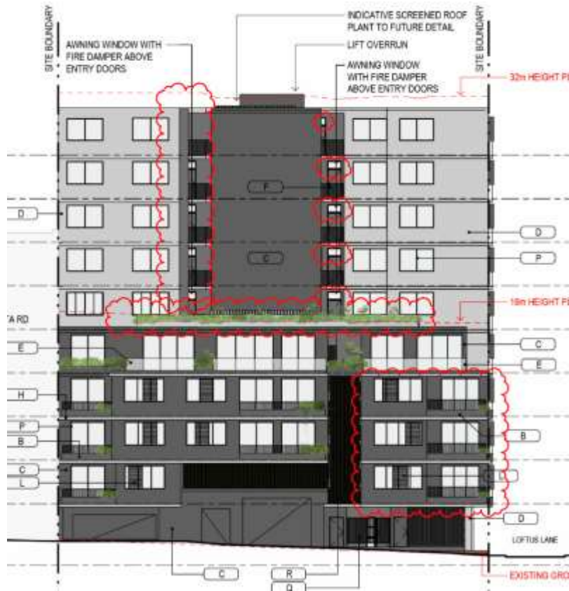
Figure 7: Extract of the proposed southern (rear) elevation fronting Loftus Lane
