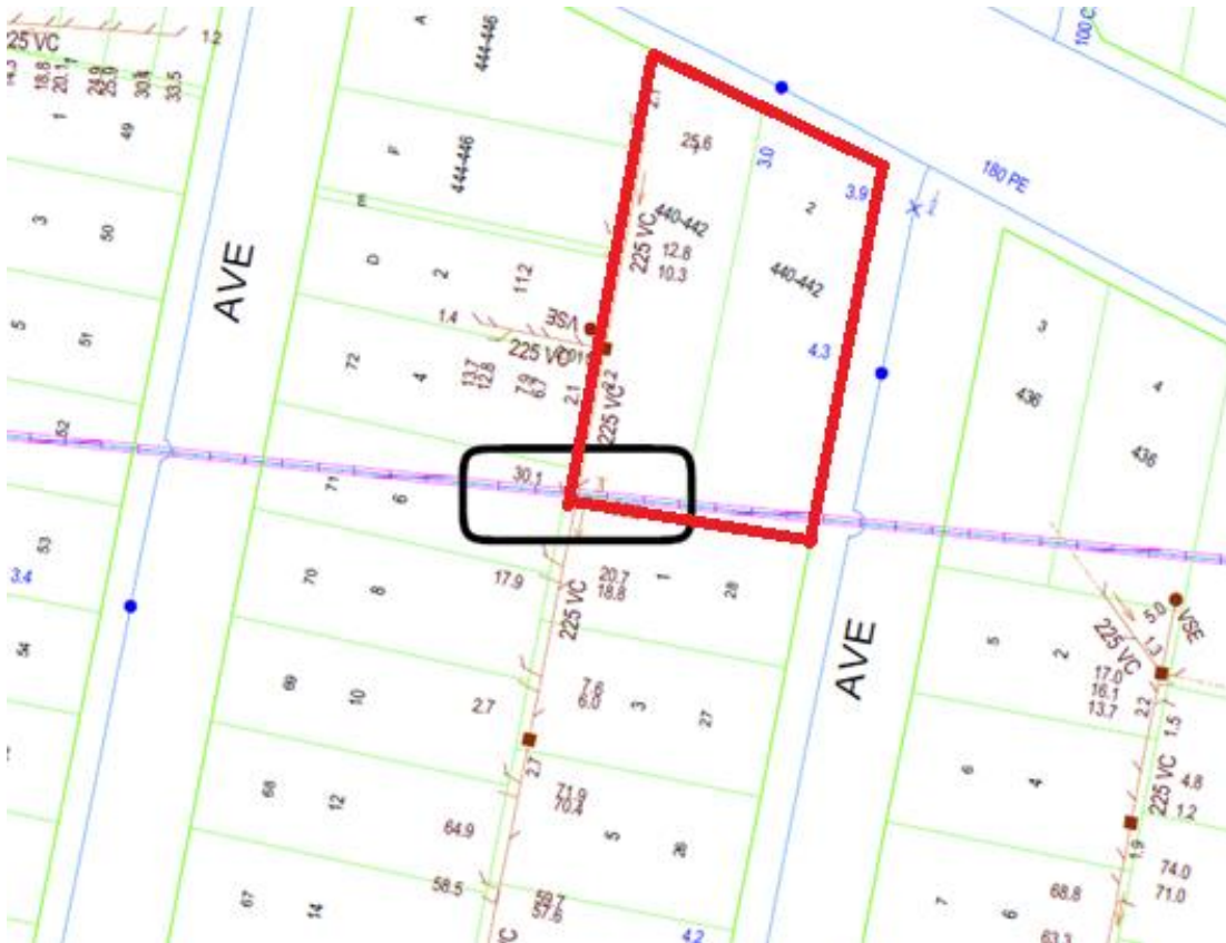
Figure 9: State Heritage listed Pressure Tunnel and Shafts (marked in purple), which traverses the site (outlined in red)
