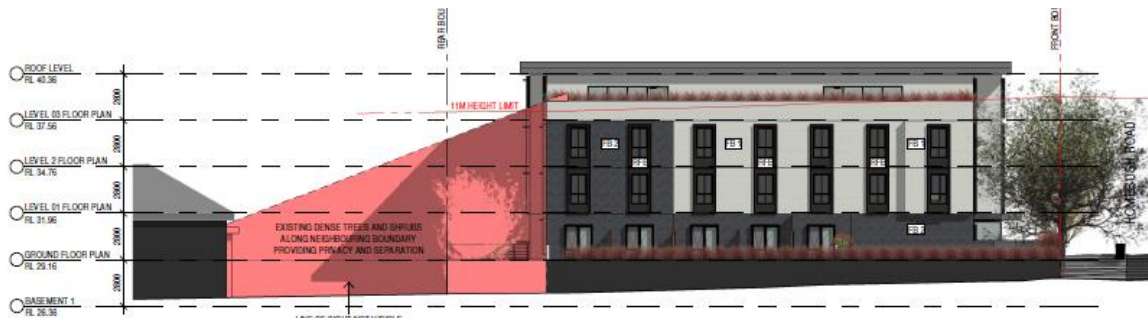
Figure 8. Amended southern elevation showing a compliant building height, three (3) storey presentation, additional external privacy screening, and incorporation of face-brick to complement the prevailing streetscape character.
