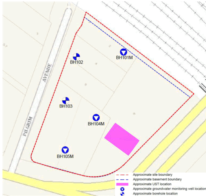
Figure 22 – Borehole and Groundwater Monitoring Locations Source: El Australia
