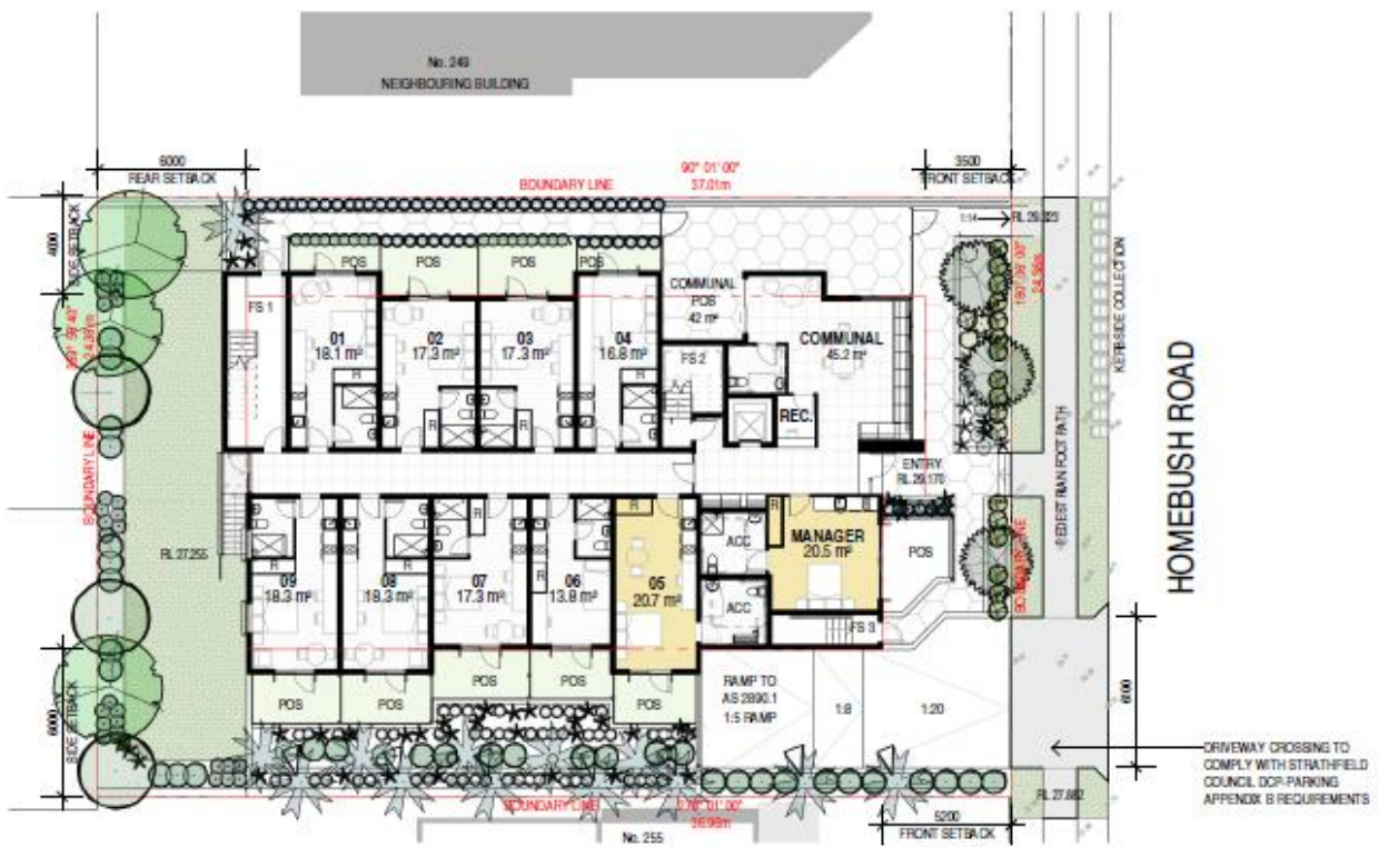
Figure 5. Amended ground floor plan showing replacement of the commercial area with a communal area, increased deep soil planting in the rear setback and increased perimeter planting on structures.
