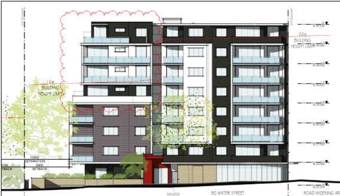
Figure 5: View of development from Water Street showing extend of non-compliance
