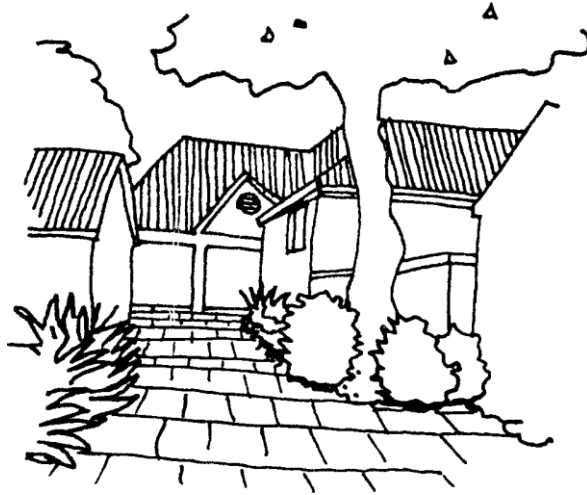
FIGURE 20: PERVIOUS AREAS ADJOINING PAVED AREAS REDUCE STORMWATER RUN-OFF
