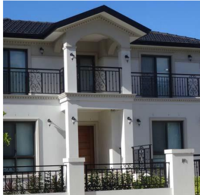
Figure A.7 - Vertically articulated two (2) storey portico provides visual prominence whilst minimising the bulk and scale of the dwelling.
