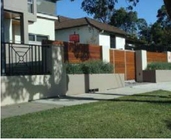
Figure A.15 – Horizontal slat or batten fences without gaps are not permitted as they do not allow passive surveillance.
