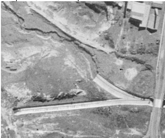
1943 Water Street diversion and concreting of Cooks River (top) and Cocks Creek (bottom). Source: SIX Maps
