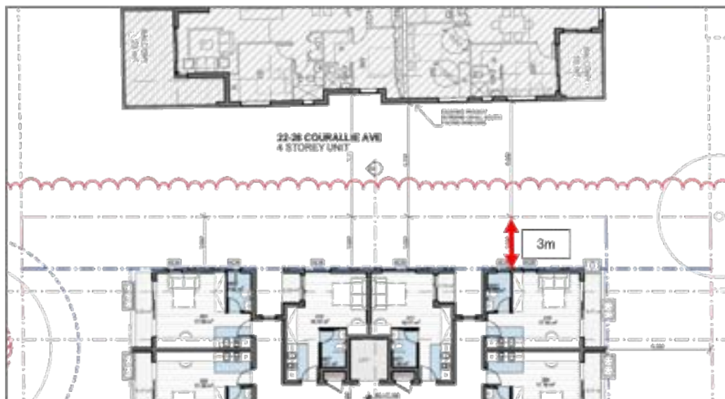
Figure 26: Level 02 Plan showing a typical northern setback interface
