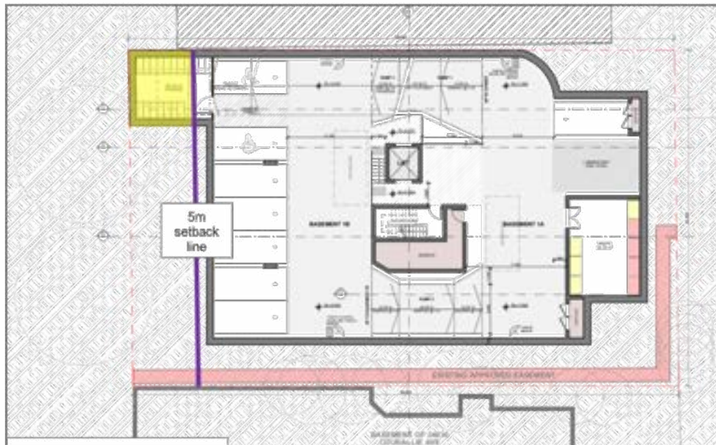
Figure 25: Basement 01 Plan showing bicycling parking underneath the driveway within the front setback (highlighted in yellow)
