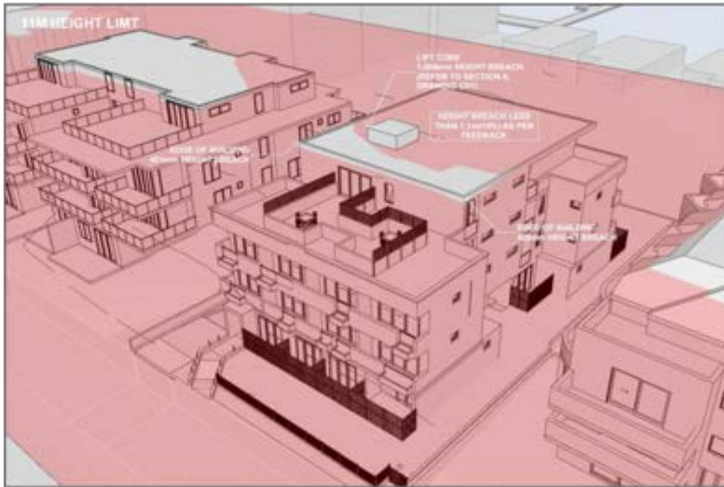
Figure 31: 3D height blanket diagram illustrating extent of breach
