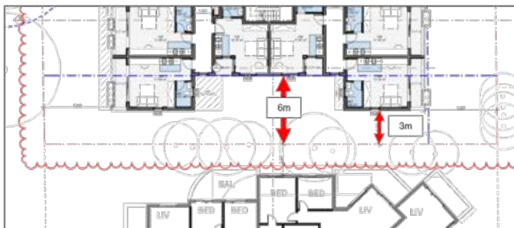
Figure 27: Level 01 Plan showing typical southern setback interface
