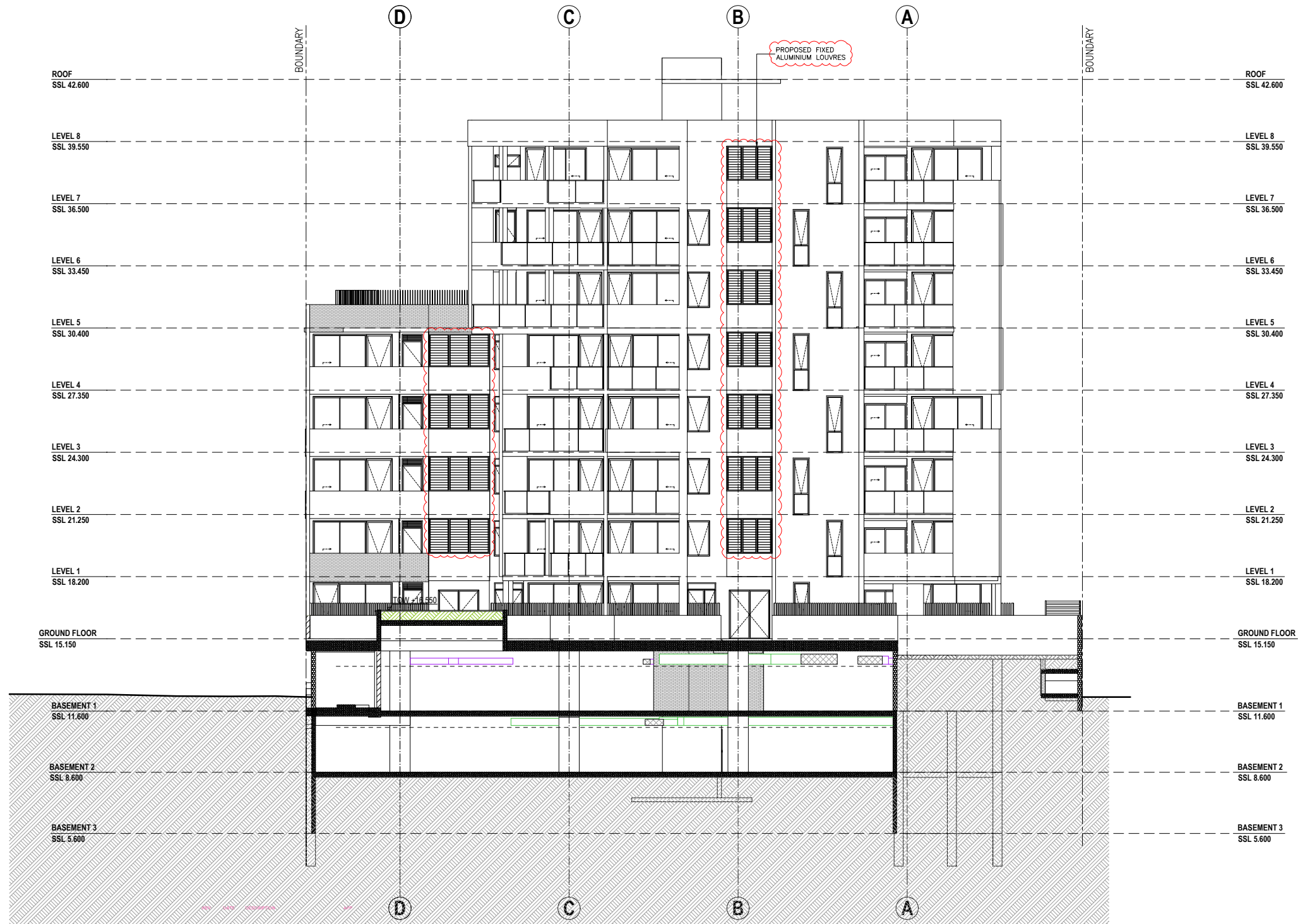
NORTH ELEVATION BUILDING A
