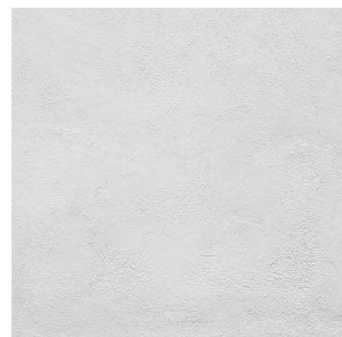
RN1 - WHITE RENDERED FINISH OR EQUIVALENT SIMILAR LOCATION: FRONT FENCE WALL, PLANTER BOXES, FIRST FLOOR BAND FEATURE, ROOF SLAB EDGE
