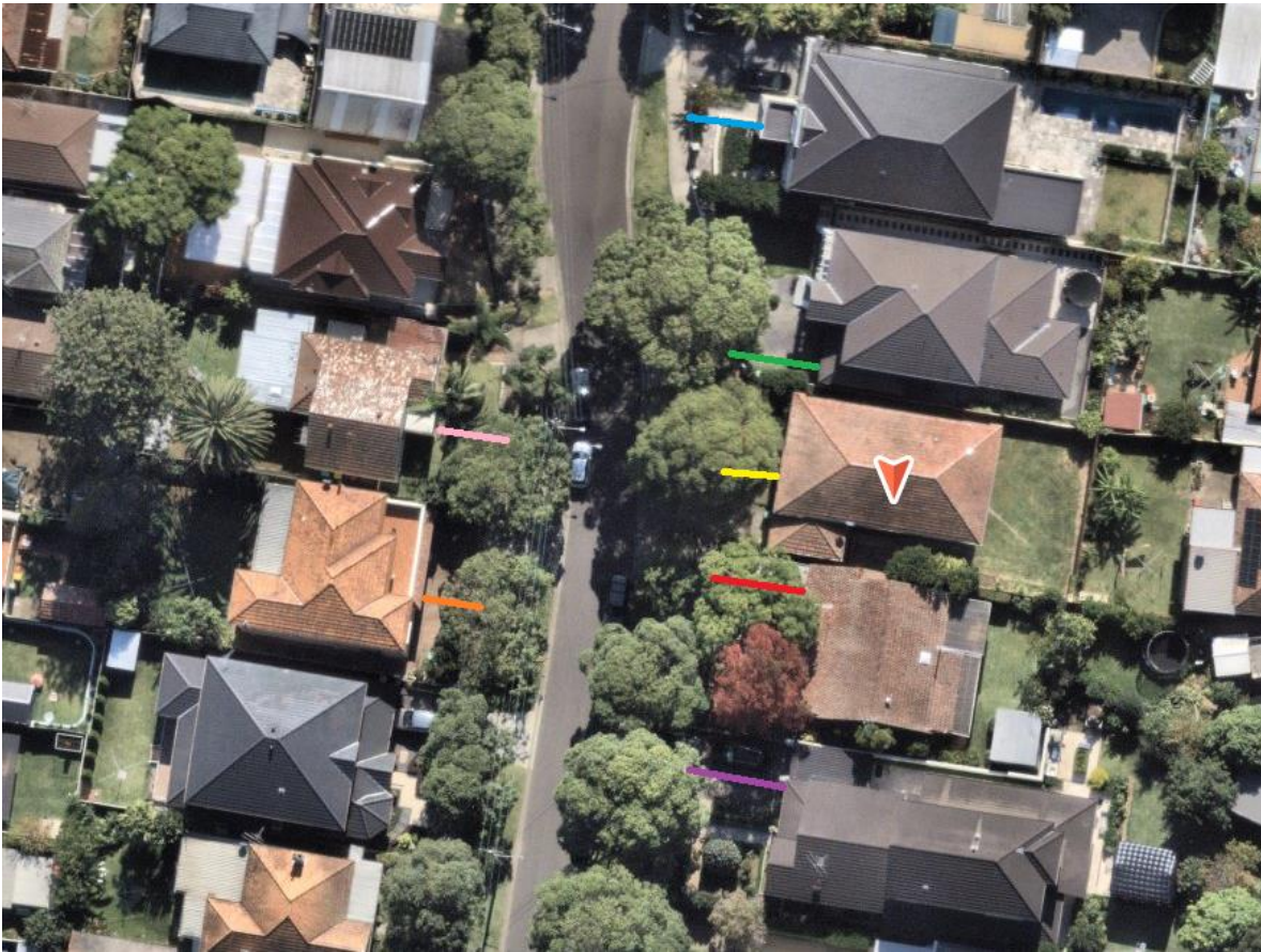
Figure 25 – Front setbacks: Yellow 4.4m (the site), Red 8.4m (14 Cross Street), Purple 9m (16 Cross Street), Green 7m (10 Cross Street), Blue 6.5m (8 Cross Street), Pink 5.5m (13 Cross Street), Orange 4.4m (15 Cross Street).
