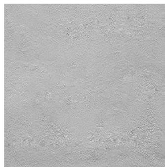
RN2 - NATURAL LIGHT COLOURED RENDERED FINISH OR EQUIVALENT SIMILAR (TO MATCH BL1) LOCATION: NORTH & SOUTH GROUND FLOOR SIDE WALLS
