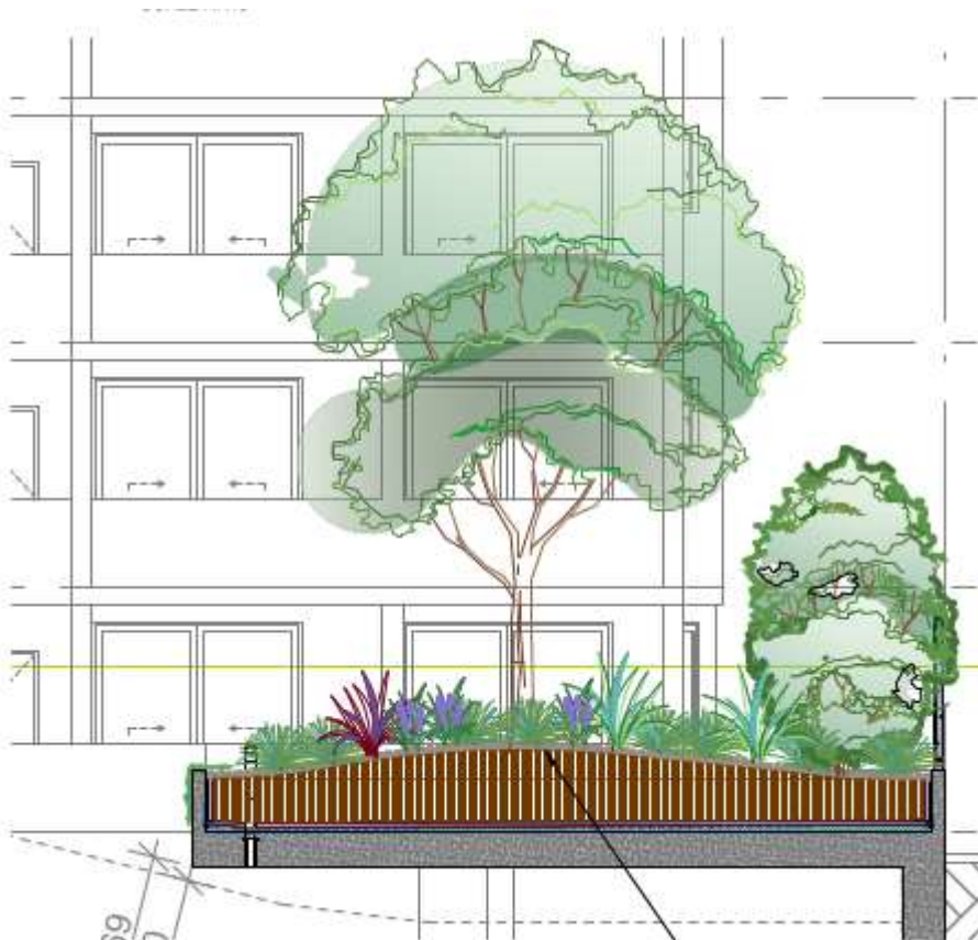
Figure 34. Extract of the landscape plan showing the proposed 10m mature height tree at the rear only providing visual privacy attenuation to the 1 st three levels.
