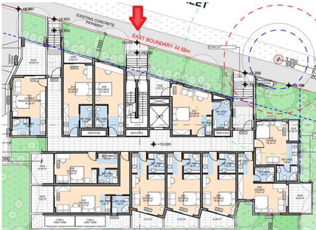
Figure 32. Extract of the ground floor plan, highlighting the stairs entry that service levels 1-4 but not the ground floor units.
